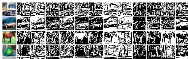
Fig. 3. Each row shows an example image from CIFAR10 (column 1) and the corresponding output of 12 typical transduction filters (columns 2–13).
